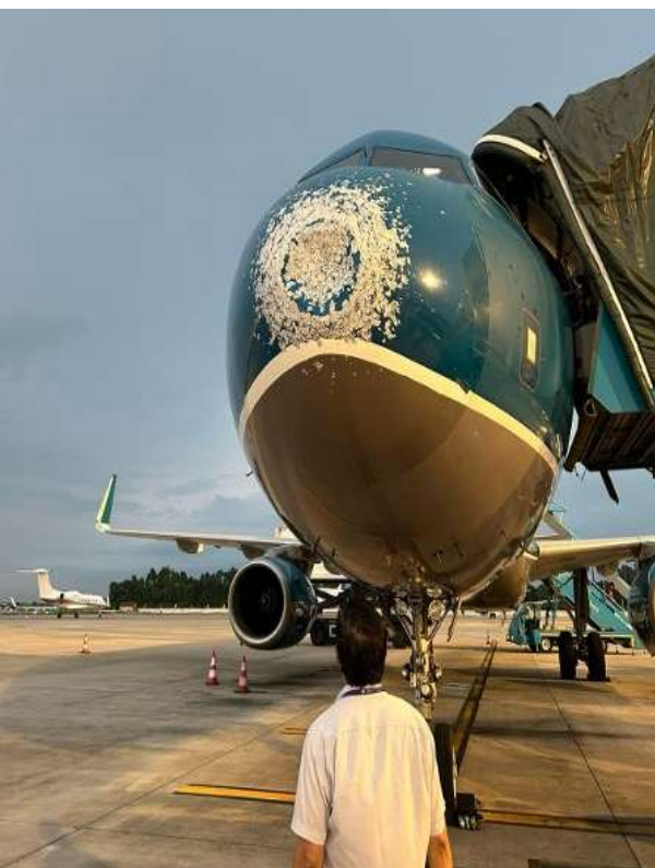
AIR TURN BACK DUE TO THE WINDSHIELD BROKEN WHILE FLYING THROUGH A BAD WEATHER AREA HVN1207 HAN-VCA MAY.2024
